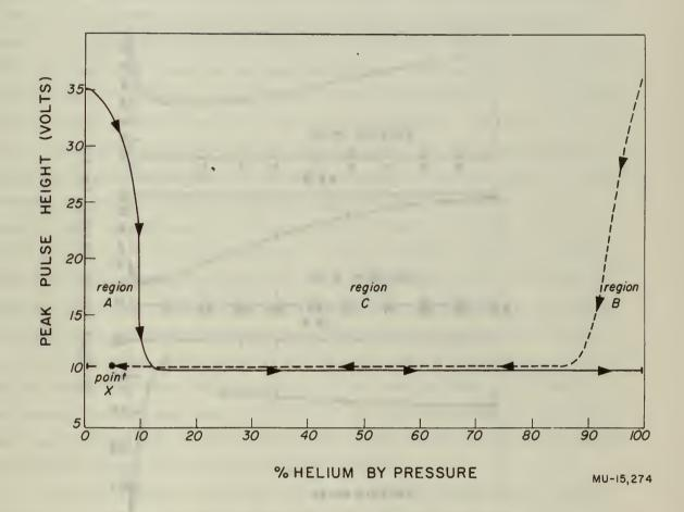
Fig. 10. Relative pulse heights, A-He mixtures. Cm 244 source. 40 psi total pressure.
